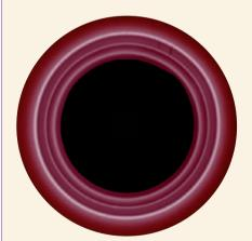
Liesegang rings are circular patterns formed by ions precipitating in well-defined areas, rather than a single place, of a gel. They are, however, formed by a relatively small number of combinations of species and supports. Most of the species are ionic and offer little chance to tune their properties such as size or solubility, so the rings are generally not controllable.
