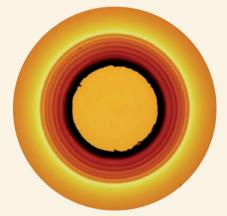
to create more predictable Liesegang rings (pictured; *J. Am. Chem. Soc.* **132**, 58–60; 2010). A sheet of agarose gel was soaked in a solution of similarly charged nanoparticles. A disc was then cut from the middle of the sheet and filled with a solution of the oppositely charged nanoparticles. As these diffuse through the gel over a day or more, they form rings of precipitate of equal amounts of nanoparticles of both polarities.
