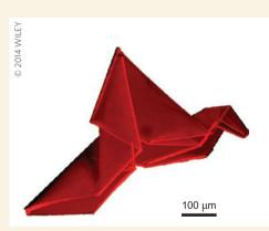
the two PpMS layers using photolithography results in folding of the material at those lines — and whether the gap is in the top or bottom film determines the direction of the fold. The radius of curvature of the fold is determined by the width of the gap, with folding angles between 0 and 180° possible.
