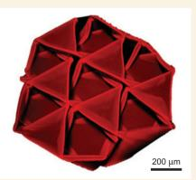
around 1 mm. As the PNIPAM becomes hydrophobic above a certain temperature, the hydrogel contracts on heating — this phenomenon means that the origami can be reversibly unfolded and refolded. One limitation of the material is that all folds occur at once, rather than being able to fold along the patterned lines in a specific order. Nonetheless, this approach could be used to form structures or small-scale soft robots with function as well as beauty. CH
