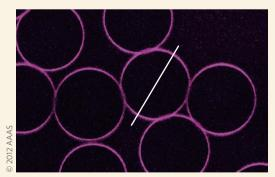
central cavity. Aqueous solutions of CB[8], gold nanoparticles functionalized with electron-deficient aromatic ligands, and a water-soluble polymer with electronrich naphthol side chains were prepared. These were then flowed into one arm of a T-junction in a microfluidic device. Oil flowing perpendicularly to the aqueous stream sheared off microdroplets containing the three building blocks, which then assembled into hollow microcapsules as the polymer
