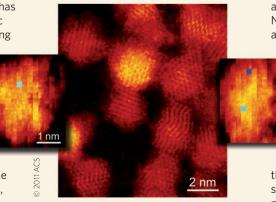
that a combination of electron energyloss spectroscopy (EELS) and annular dark-field scanning transmission electron microscopy (ADF-STEM) can be used to image manganese dopant atoms buried within zinc selenide nanocrystals. First, using Nano Lett. 11, 5553-5557 (2011)
