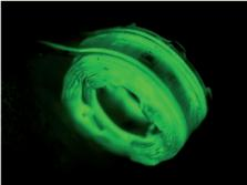
in microfluidics, making the resulting SU-8/PDMS networks well suited to fluid transportation. The transport of a green and a red dye (fluorescein and Rhodamine B, respectively) through a dual-channel cylindrical device was clearly observed by fluorescence. Furthermore, the devices are biologically inert and remain curved in cell culture media, which means they are promising for bio-applications. AP
