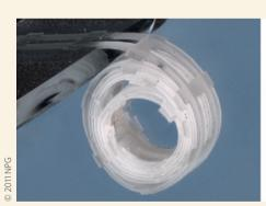
with the original solvent. The curving can be precisely controlled by the UV exposure, film morphology and heating conditions, which enabled the researchers to assemble various differently curving segments into complex three-dimensional architectures.
