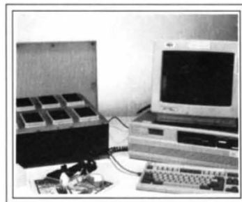
Figure 2. Amino acid indexer. The prototype is capable of simultaneous synthesis of 960 peptides on 10 microtiter plates.
