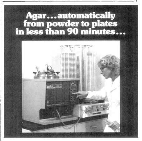
Up to 8 liters (400 plates) of high-quality agar whenever you need it Any laboratory can have high quality agar whenever it's needed thanks to two benchtop instruments — the Agar-Matic, an 8 liter sterilizer, and the PourMatic, a self-stacking carousel-type petri dish filler.
