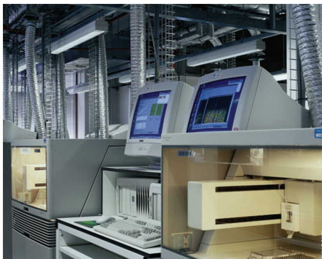
Next-generation sequencing is already several orders of magnitude more efficient than the Sanger capillary-array electrophoresis (CAE) machines that were the workhorse of the Human Genome Project.
