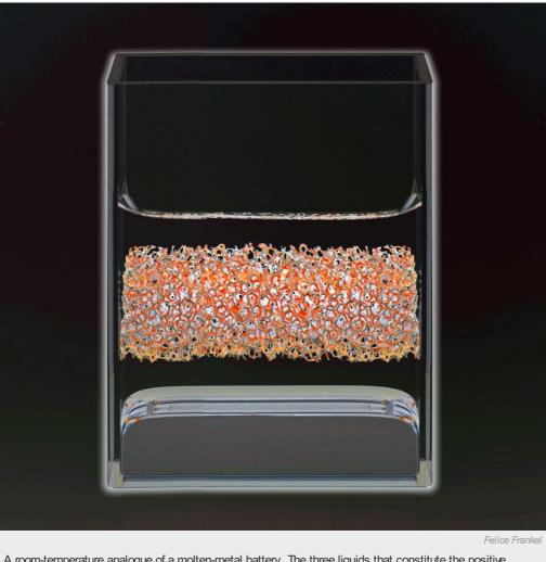
A room-temperature analogue of a molten-metal battery. The three liquids that constitute the positive electrode (bottom), the electrolyte (middle) and the negative electrode (top) stay separated like oil and vinegar.
