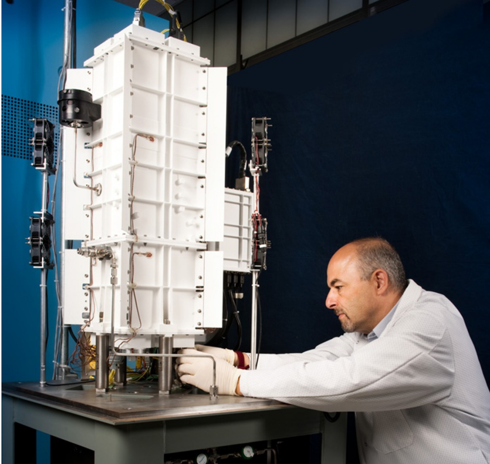
The Advanced Stirling Radioisotope Generator would have used one-quarter of the plutonium needed for existing NASA power sources.
