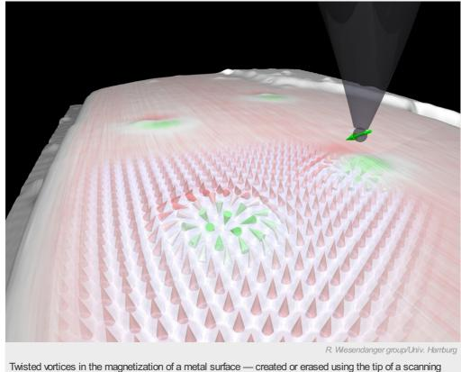
Twisted vortices in the magnetization of a metal surface — created or erased using the tip of a scanning tunnelling microscope (STM) — could provide a new way of recording data.
