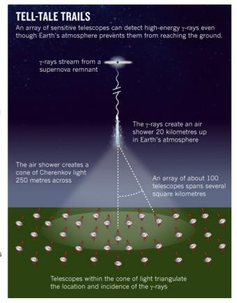
The CTA would have the energy range, sensitivity and angular resolution to find many more. It would consist of two sites, one in the Northern Hemisphere and one in the Southern, each with dozens of telescopes spread over about ten square kilometres. Together, they could identify an estimated 1,000 high-energy γ-ray sources. With a construction start in 2015, the facilities are projected to carry a price tag of €200 million (US\$268 million).
