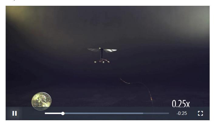
A robot as small as a housefly has managed the delicate task of flying and hovering the way the actual insects do.
