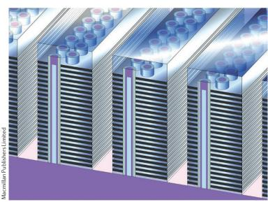
of the structure," says Ma. Most commonly, these defects are voids buried in the stacks, which may cause an open-circuit failure, and W bridges between wordlines, which may cause short-circuit failure. Also, W residues at the bottom of the slits between the wordlines and failure of substitution to give a W-SiO<sub>2</sub> layer are other sources of defects in the devices.
