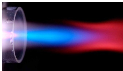
A plasma torch. Adapted from Aeschliman, D.B. et al. , J. Anal. At. Spectrom. 18 , 1008-1014 (2003), with permission of the Royal Society of Chemistry.
