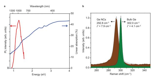
Figure 2 (a) Absorption (blue) and PL (red) curves. (b) Raman spectrum (brown) with a Lorentzian fit (dashed line) giving the position and width as indicated. For comparison, the bulk germanium spectrum is shown in green. The shift of the peak is due to quantum confinement.<sup>25</sup> NC, nanocrystal; PL, photoluminescence.
