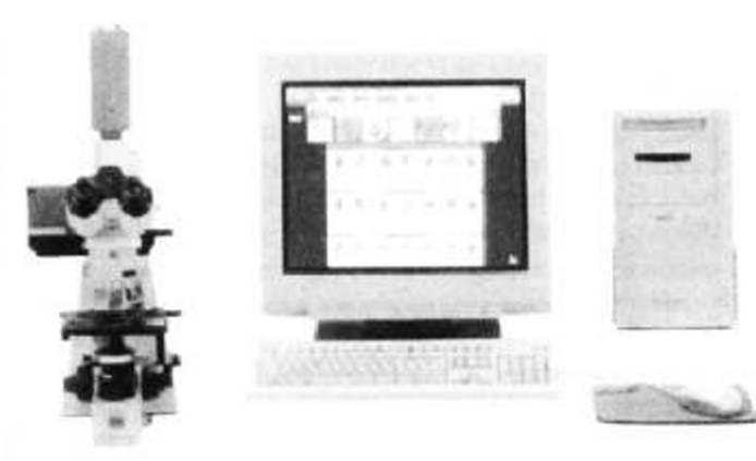
Fig. 1 The teleconsultation system that was used to capture metaphase images and karyotypes included a photomicroscope, CCD camera, and a Macintosh PowerPC with Perceptive Scientific Instruments software.
