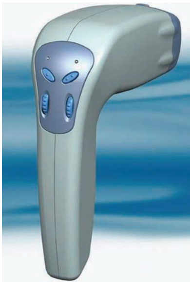
Figure 1 Image of the hand held, portable digital slit-lamp (PSL) video camera developed at the Lions Eye Institute (LEI) in Perth, Western Australia. This hand held instrument has a fixed width slit beam with two selectable alignments. A third 'red reflex' coaxial illumination is also selectable.
