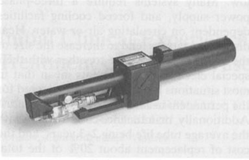
Fig. 1. Hand-held version of diode laser, utilising a direct ophthalmoscope.
