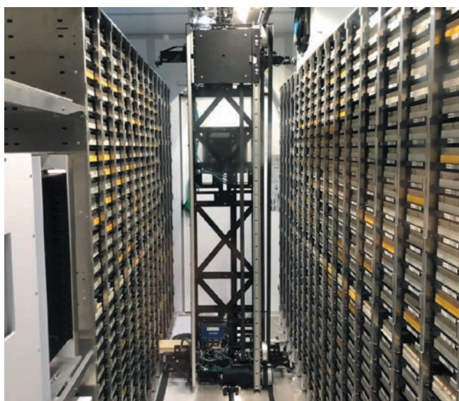
▲ Auto-storage for dimethyl sulfoxide solution of compounds in 2D barcoded tubes stored at -20 °C.
