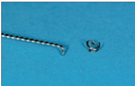
Fig 3. Endodontic file used to retrieve fractured thread
