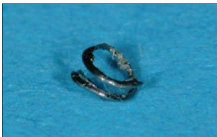
Fig 4. Fractured thread removed from implant
