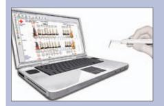
The Florida Probe System exploits the power of a PC to create a probing unit enabling constant force, standardised measurements and multi-lingual voice call-outs. A sole operator can complete a comprehensive examination in less than 12 minutes, and then present the patient with a printed report to take home with full details of his or her periodontal disease.
