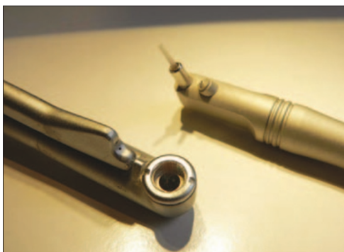
Fig. 15 Older (left) non-contact and newer (right) laser hand-piece with sapphire contact tip. The older head incorporates a flat sapphire window
