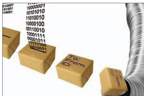
Fig. 2 The IP (Internet protocol) breaks data down into small packets which are labelled before sending off into the Internet. The TCP (transmission control protocol) then deals with the delivery of the packets to the correct destination
