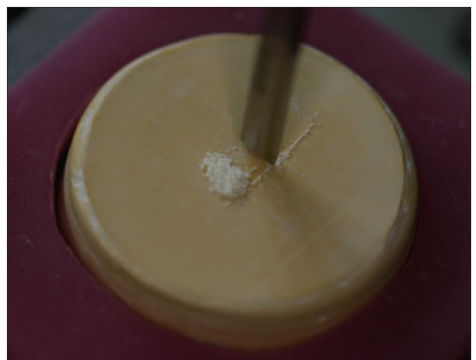
Fig. 5 Photograph of specimen during abrasion testing
