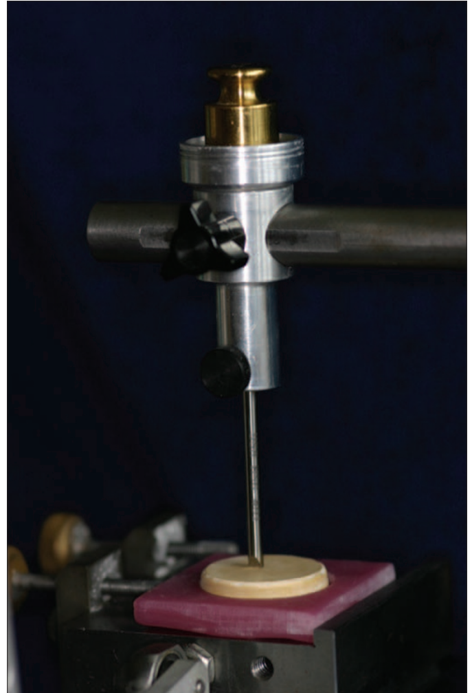
Fig. 4 Photograph of abrasion device with 50 g weight applied
