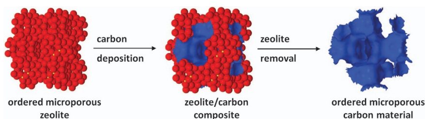
Figure 1 Schematic illustration of the templating process in which first carbon (indicated in dark blue) is deposited onto the pore walls of the zeolite structure (oxygen atoms of the structure indicated in red), followed by an additional heating step and removal of the zeolite, resulting in an interconnected ordered microporous carbon structure.
