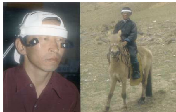
Figure 14 Miniature UV sensors worn on a headband throughout daily activities.
