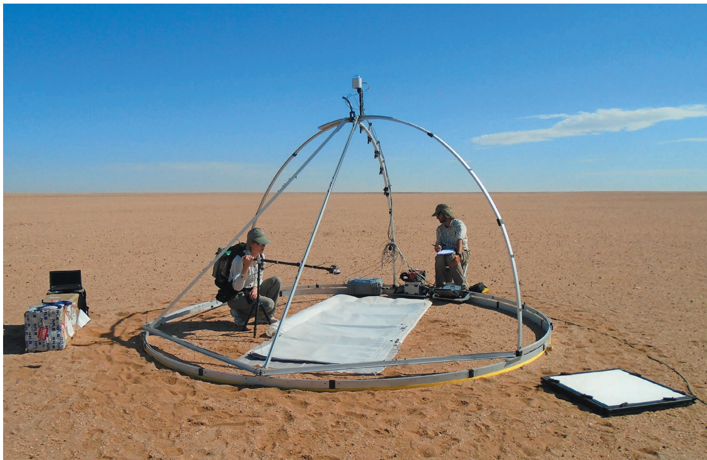
Ground-based measurements of light bouncing off deserts can be used to calibrate satellite observations of reflectivity and improve climate modelling.
