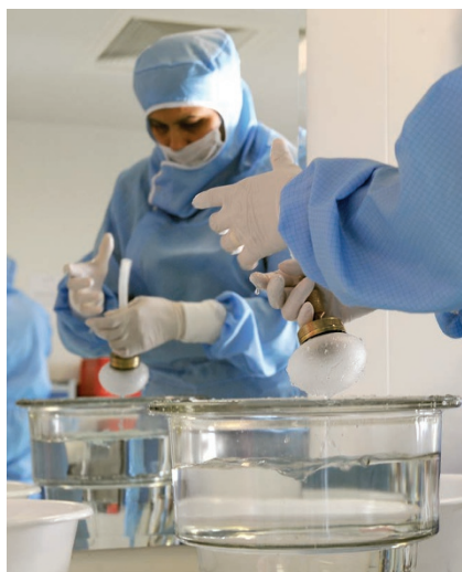
Silicone membranes for breast implants are tested for water resistance.
