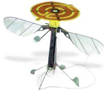
buildings. The top of the device has a patch containing copper electrodes. Switching on the voltage between the electrodes induces opposing charges on the surface of a nearby target, generating an electrostatic attraction. Switching off the voltage releases the robot. The device can cling to a variety of surfaces, including glass, wood and leaves.
