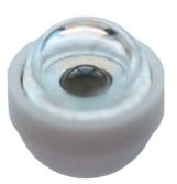
the cups to a stretched silicone polymer sheet, the authors shaped the array into a retinalike dome (pictured). The cups concentrated incoming light, boosting the sensitivity of the eye by more than three times compared to cameras that did not use this device.
