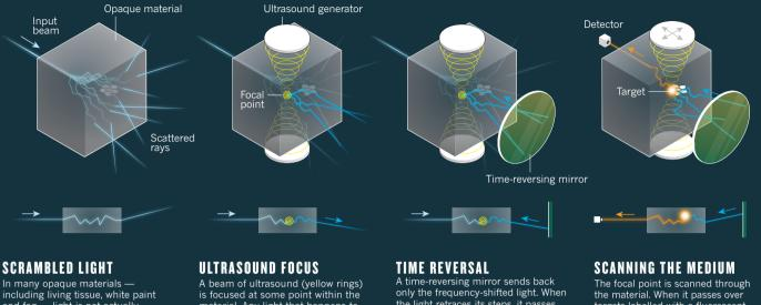
In many opaque materials including living tissue, white paint and fog — light is not actually absorbed. It simply bounces around in the material until it is too scrambled to form an image. A beam of ultrasound (yellow rings) is focused at some point within the material. Any light that happens to bounce through this point will undergo a slight shift in its frequency (blue rays).
