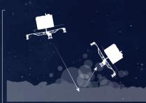
The surface is too hard and Philae bounces. The surface is too soft and the lander struggles to secure itself with harpoons and screws. Low gravity makes drilling difficult.
