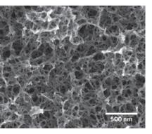
honeycomb-like structure (pictured) that has excellent electrical conductivity, unlike most other self-assembled organic-inorganic systems. The team studied the material only in bulk form, but say that the results could be even better if the polymer was in two-dimensional sheets, perhaps leading to more efficient solar cells and supercapacitors. J. Am. Chem. Soc. http://doi.org/ spj (2014)
