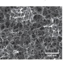
honeycomb-like structure (pictured) that has excellent electrical conductivity, unlike most other self-assembled organic-inorganic systems. The team studied the material only in bulk form, but say that the results could be even better if the polymer was in two-dimensional sheets, perhaps leading to more efficient solar cells and supercapacitors.
