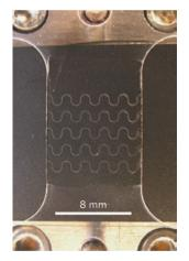
interlocking channels that are criss-crossed by proteins holding the structure together. The researchers etched similar patterns into glass (pictured) and filled in the gaps with shock-absorbent polyurethane, creating a material that is 200 times tougher than standard glass.
