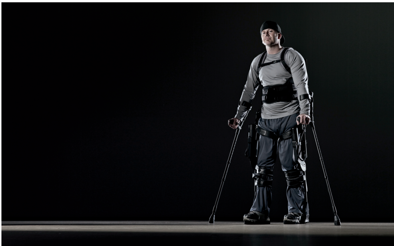
Paul Thacker, who was paralysed from the chest down in a snowmobile accident, can walk again using an exoskeleton that has four motors and 15 sensors.
