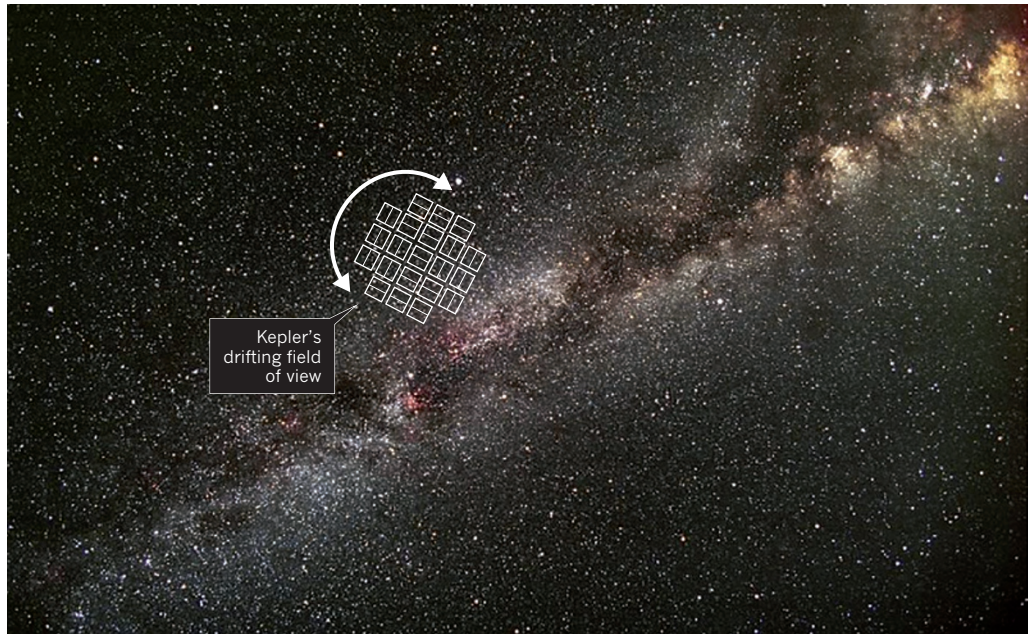
Kepler’s field of view is now drifting because of a failure of two of its four reaction wheels.
