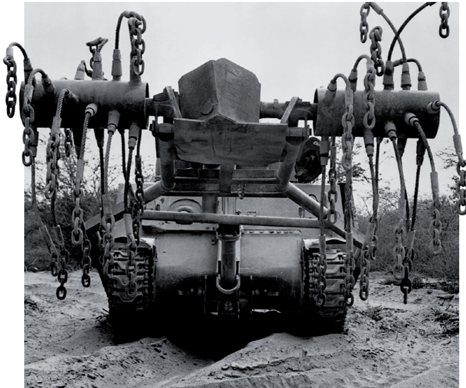
A Second World War Marine M-4 tank carries a mine detonator installed by the US Navy Seabees.
