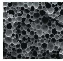
create porous polystyrenebased foams (**pictured**). By incorporating various other polymers into their foams, the researchers controlled the surface topology of the pores and thus the distribution and size of the places where cells and proteins could attach over three dimensions.
