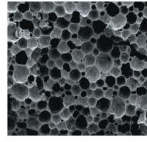
create porous polystyrenebased foams (pictured). By incorporating various other polymers into their foams, the researchers controlled the surface topology of the pores and thus the distribution and size of the places where cells and proteins could attach over three dimensions.
