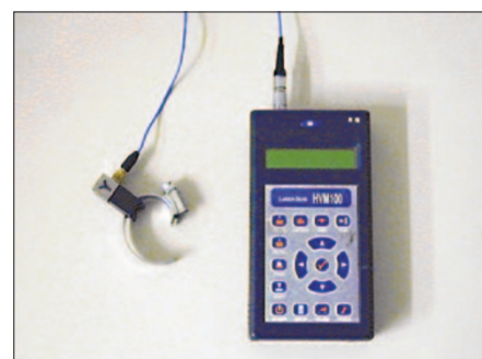
Fig. 2 Typical equipment used for measurement of occupational vibration exposures comprising a tri-axial accelerometer, mounting clip and human vibration meter. Such equipment is able to measure, frequency weight and provide data to enable calculation of A(8) values.
