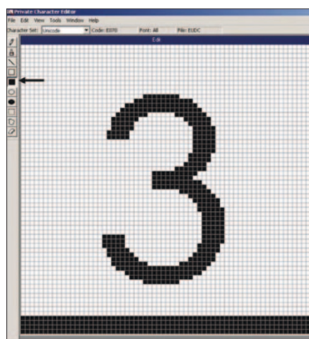
Fig. 5 The PCE editing grid; the arrow shows the filled rectangle tool, which has been selected and dragged over the requisite number of pixels to insert the underline. The number '3' has first been pasted into the grid by using the 'Copy Character' function, which is accessed via the 'Edit' menu.
