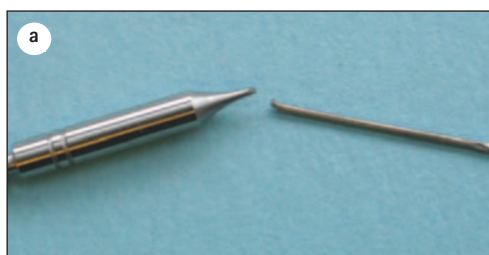
Fig. 11 A Gates–Glidden bur which fractured during use in the root canal, showing the normal point of separation, permitting removal with Steiglitz forceps. However, b) shows that this is not always the case.
