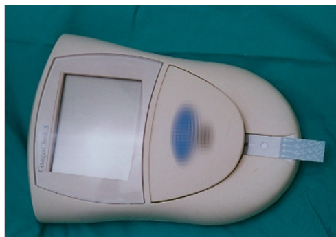
Fig. 5 The INR can be measured at the chair side by portable machines that require only a finger-prick blood sample
