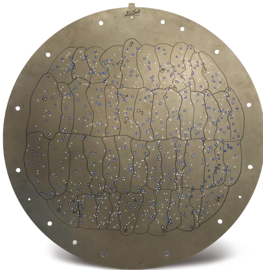
Holes in aluminium plates channel light from individual galaxies to calculate how fast each is receding.
