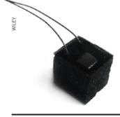
The device consists of carbon nanotubes — which heat up when exposed to laser light — wrapped in a polymer and dispersed in silicone. The heat warms one side of the converter more than the other, and the flow of heat to the cooler side generates an electric voltage.
