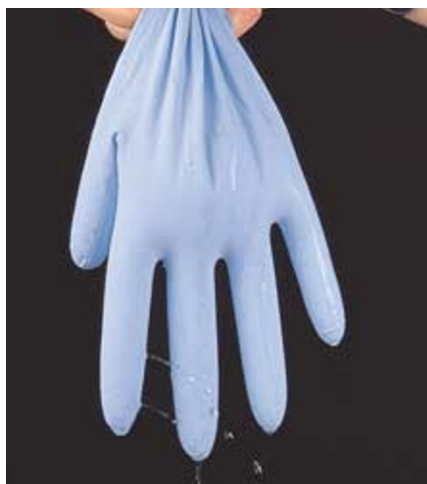
Fig. 1 Water inflation method for puncture detection
