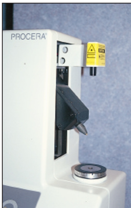
Fig. 4 Scanner machine with die in situ
