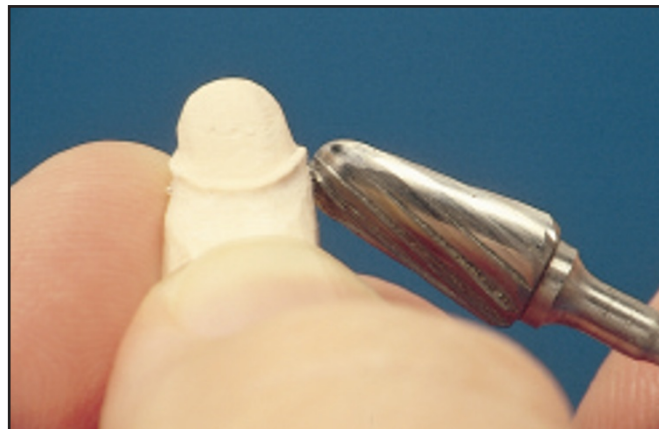
Fig. 3 Trimmed die ready for scanning
