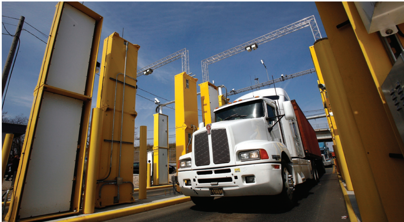
Advanced Spectroscopic Portals developed by the US Science and Technology Directorate scan vehicles for radioactive material.
